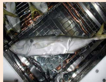
Horse mackerel under alcohol brine freezing at -25^{\circ}\text{C}
