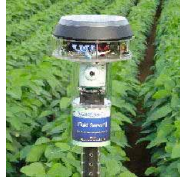
Field Server robot that measures and monitors fields
