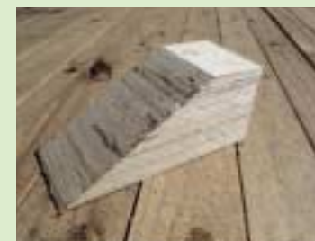
①采用LVL(laminated veneer lumber)的楔子(档木)
