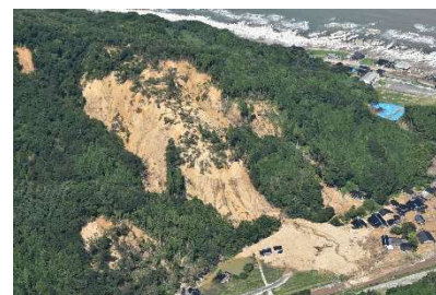
Hillside failures areas due to earthquakes and heavy rains (Suzu City, Ishikawa Prefecture)
