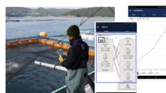
Aquaculture control cloud system Feeding data and other information related to culture management are given as input through a tablet and the data is integrated in real time by cloud management. (Photo by Fisher's cooperative of Azuma-cho and Minaminohon Information Processing Center)
