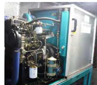
Power generator using a mixture of biogas and BDF
