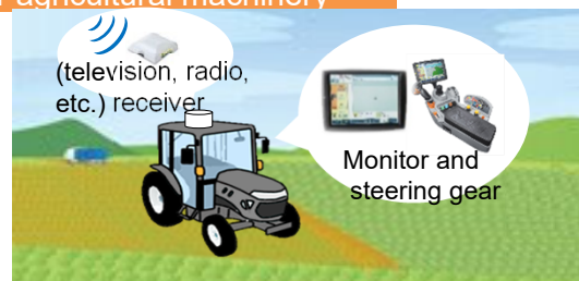
Promoting the spread of "automatic steering systems" that enable highly accurate work and contribute to energy conservation by reducing duplication of work
