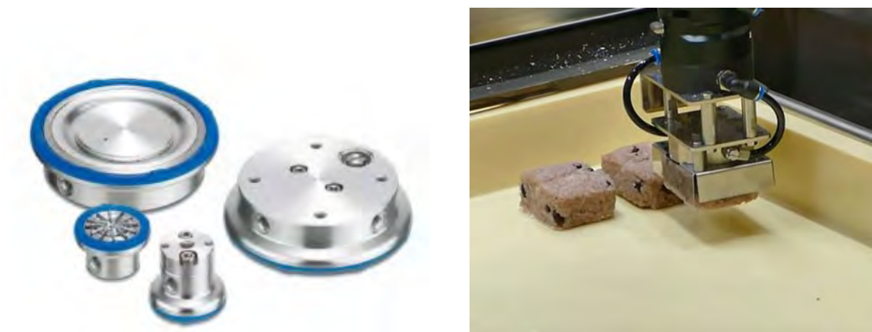
Figure 4-10: Sample non-contact suction-type robot end effector and its implementation at a food manufacturing facility
