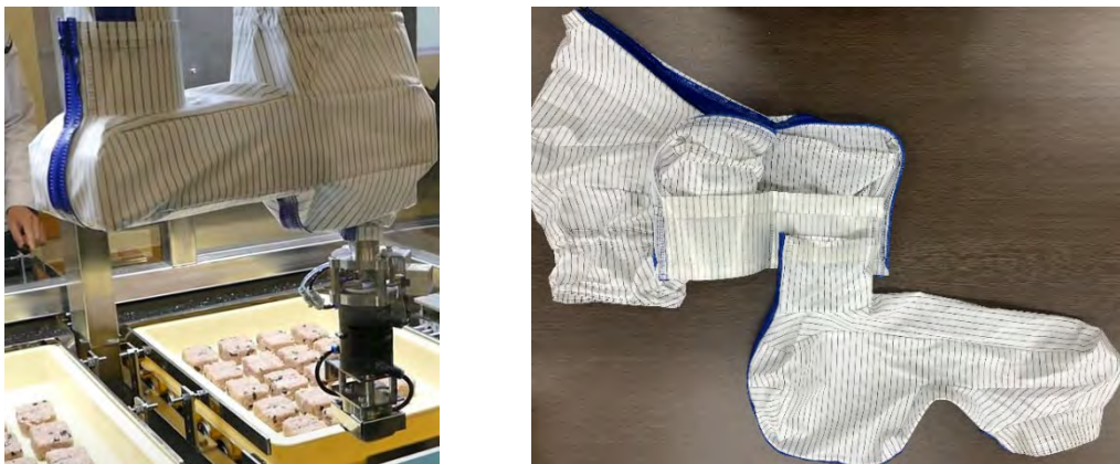
Figure 4-9: Robot protective jacket for food processing installed on a ceiling-mounted robot and the robot protective jacket removed
