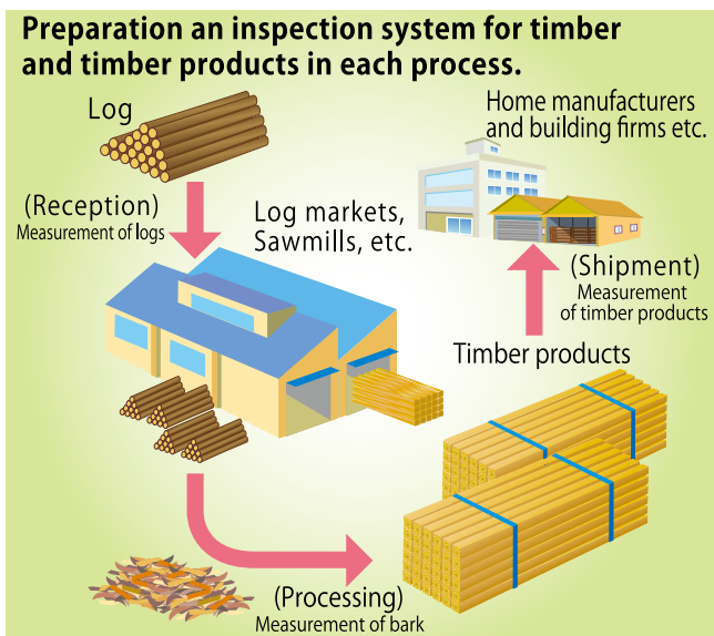
[Figure 1] Development of an Inspection System for Raw Timber and Timber Products
