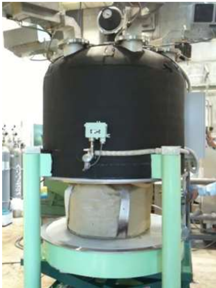
Vacuum Microwave-assisted steam distillation 減圧マイクロ波水蒸気蒸留装置
