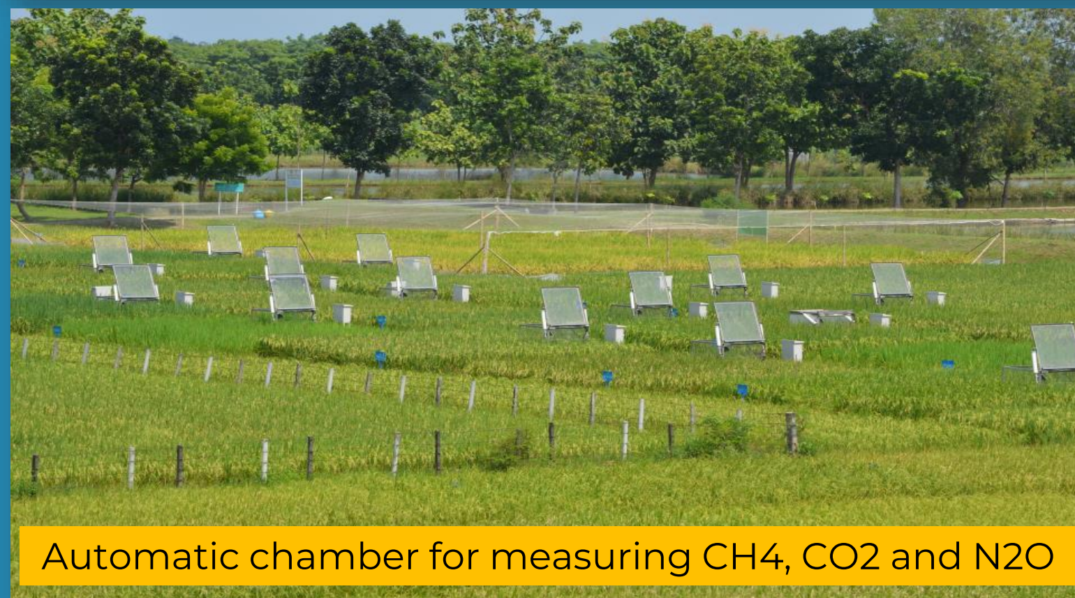
Automatic system for measuring CH 4 , CO 2 and N 2 O
