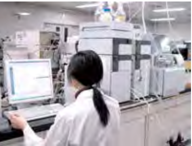
Analysis of mycotoxin contained in feed by using LC-MS.
