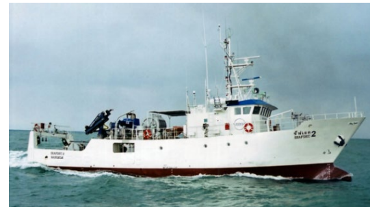
M.V. SEAFDEC 2 used for fisheries resource surveys of pelagic fish (Research vessel provided to SEAFDEC by the Government of Japan in 2003)
