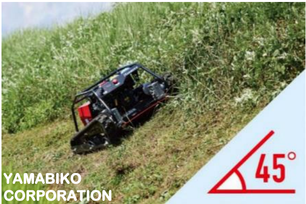
Radio-controlled mowers which can be used on steep slopes
