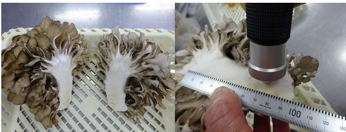
図15 子実体基部の硬さの測定 Fig. 15 Determination of hardness at the base of the fruiting body plant
