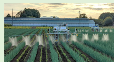
Pesticide spraying robot that can also be used for small- and medium-sized, and family-managed businesses. Source: Legmin, Inc.
