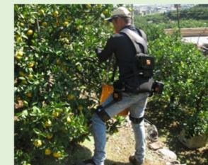
Power assist suit that can be used in hilly and mountainous areas Source: Power Assist International Corporation
