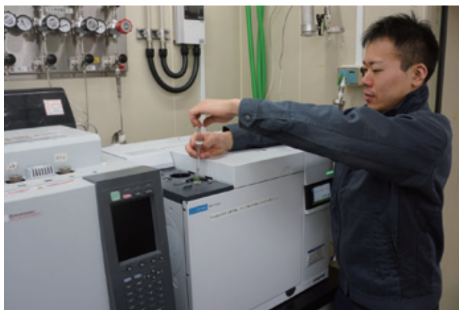
Measurement of the gas concentration of fumigants using gas chromatograph
