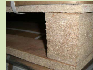
4) Pallets made of particleboard
