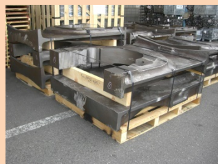
9) Wooden Pallets reinforced with Battens
