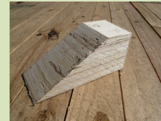
1) Wedges made of LVL (laminated veneer lumber)
